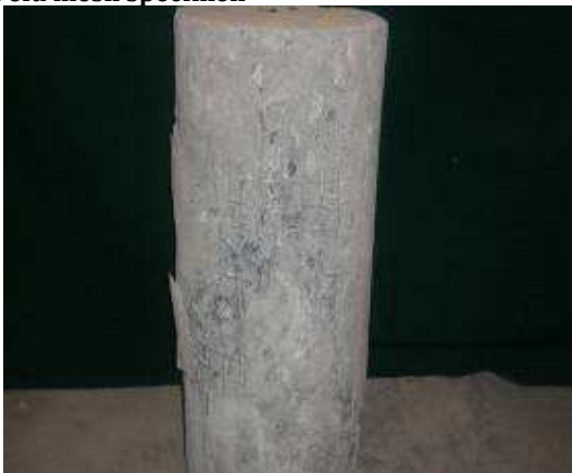
Fig. 19: Failure of GI weld mesh specimen
