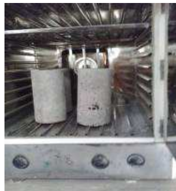
Fig. 6: Cylinders in oven @ 320°C
