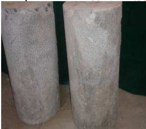
Fig. 18: Failure of Wire mesh specimen
