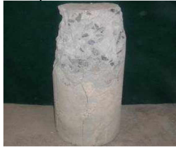
Fig. 20: Failure of Nylon mesh specimen
