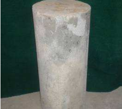
Fig. 17: Failure of glass mesh specimen
