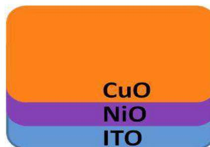
**Fig: 1 Schematic diagram of composite layers used of NiO film coated on ITO [16]**
