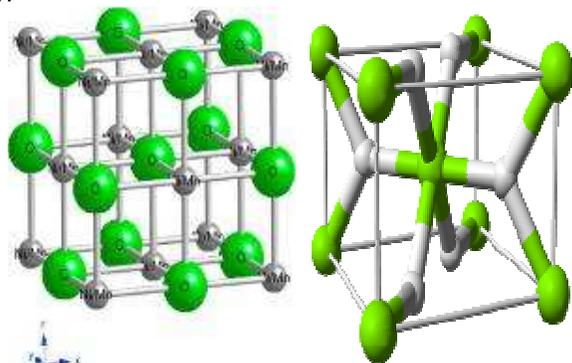
Fig: 2 Cubic structure of Nickle Oxide
