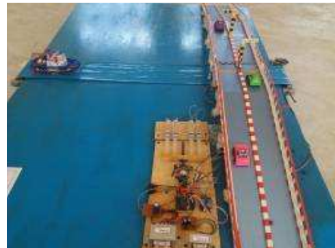
Fig.4: Result for the Condition of Green LED and Gate Open
