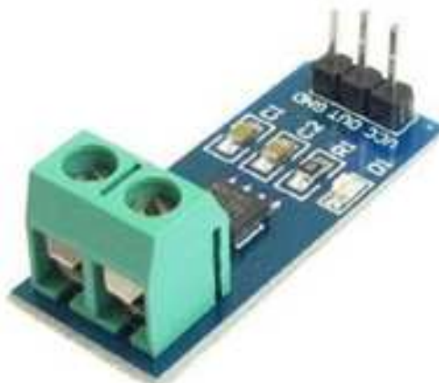
Figure 7 ACS712 Current Sensor [11]
