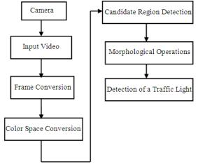
Figure2. Block Diagram of Traffic Light Detection
