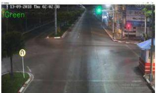
Figure7. Traffic light detection for green color
