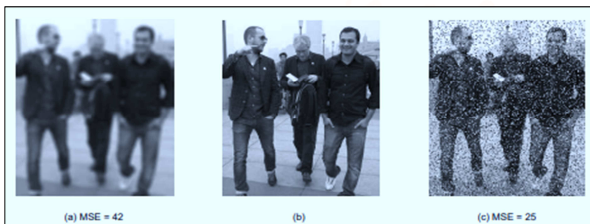
Figure 3: Original Image (b) processed with blurring in (a) and with Salt & Pepper Noise in (c)
