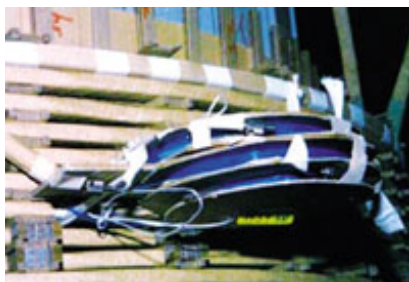
Fig.6 Temporary spooling of fiber optic sensor
