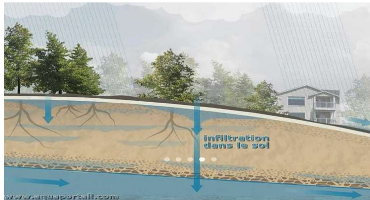
Figure 1. Water infiltration into the soil
