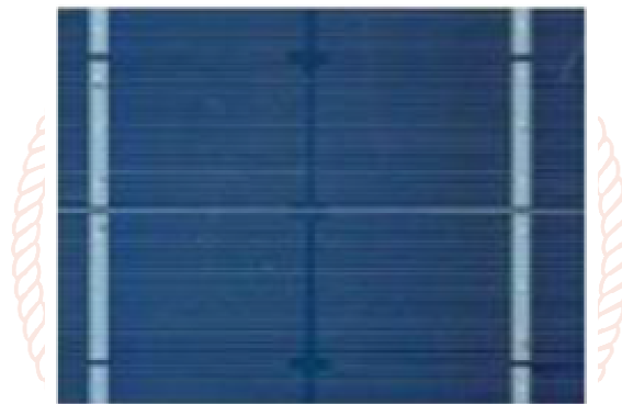
Figure 3: Single crystal cell
