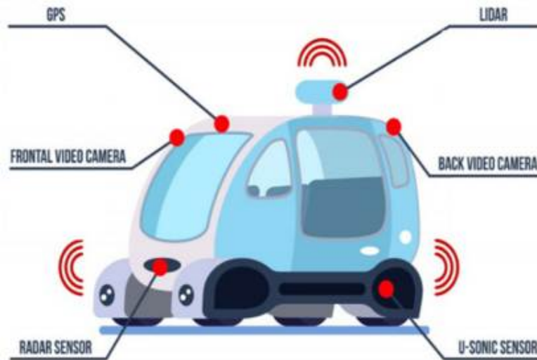
Figure 8 The main set of sensors present in an AV [13].
