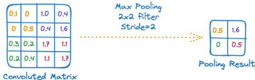
Fig5: Application of max pooling with a stride of 2 using 2x2 filter [3]
