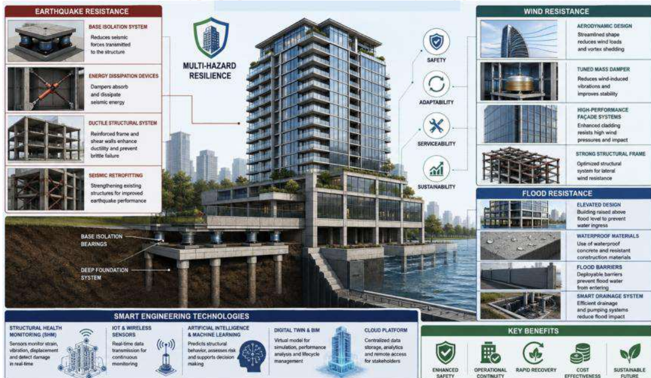
Figure 2: Multi-Hazard Resilient Building Design Incorporating Earthquake, Wind, and Flood Resistance Using Smart Engineering Technologies
