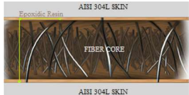
Fig. 1 Layered structure of the Hybrix material [13]
