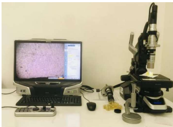
Fig. 3 The digital microscope Keyence VHX-5000
