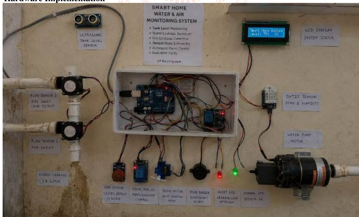
Fig. 3.1 - Complete hardware setup block diagram.
