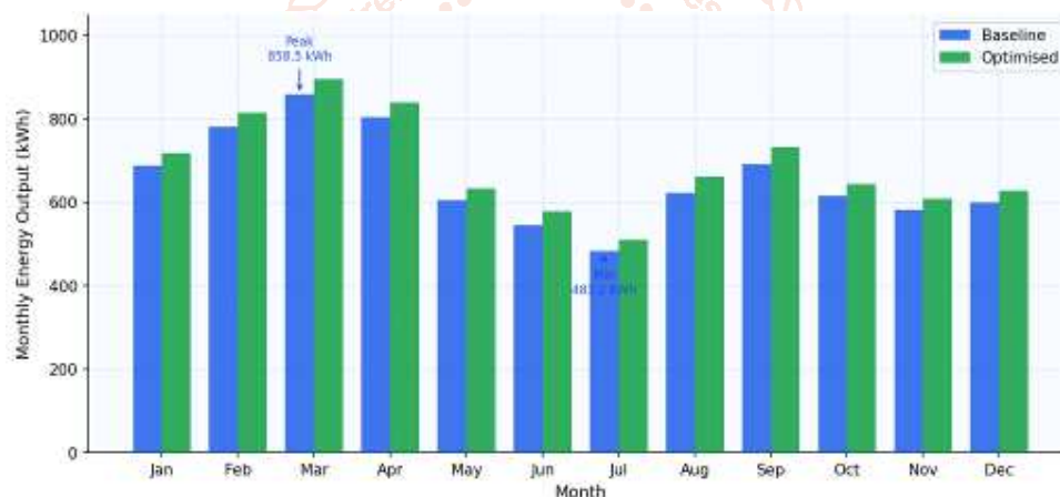
Fig. 1 - Monthly Energy Generation: Baseline vs. Optimised Output (5 kW System, Thrissur 2024)
