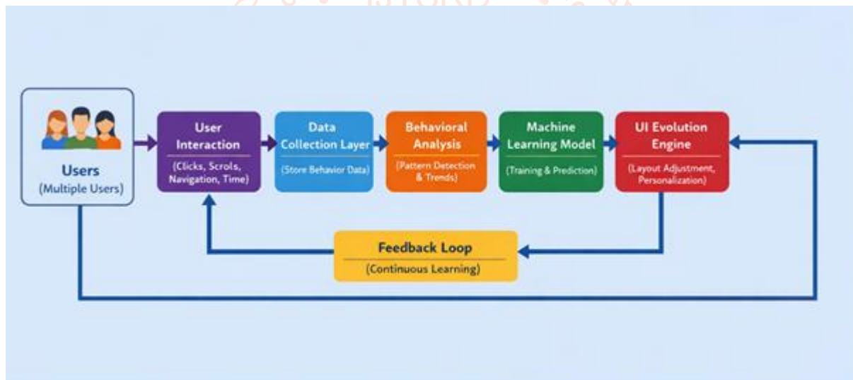
Fig. 1: Architecture of Self-Evolving User Interface using Collective Behavioral Learning
