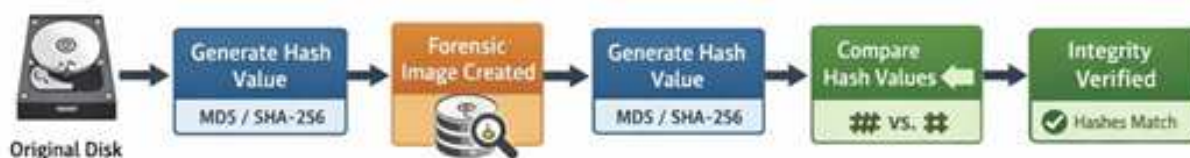
Fig.2 - Hash Verification Process in Digital Forensic Imaging
