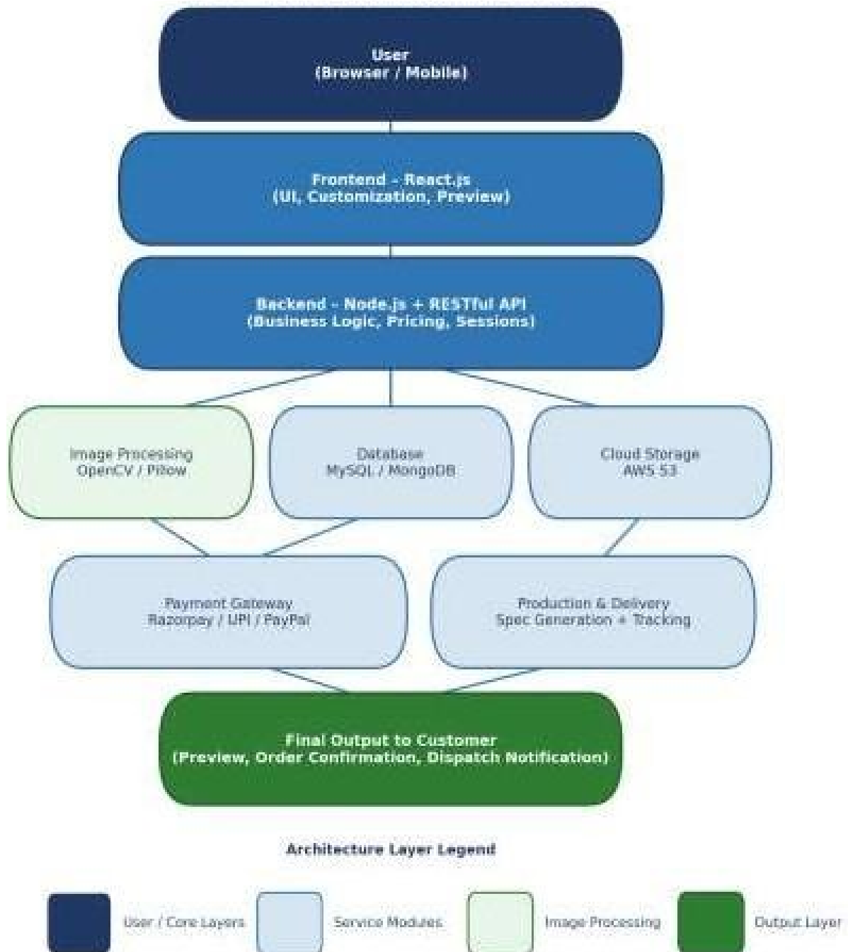
Fig. 2 — Wall Vastra System Architecture Diagram
